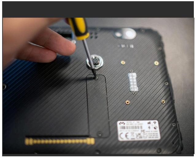
2 – Insert up to two SIM cards and one SD Card. Check the description in the chassis and push it until you feel a "click"
